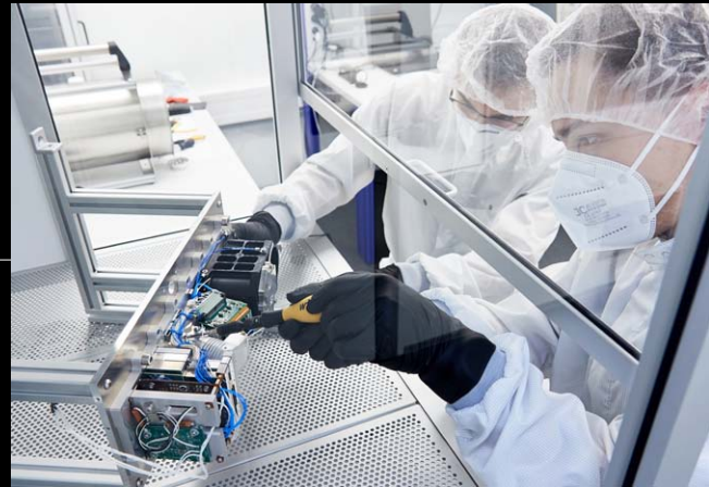
Thermal infrared camera "LiSR": The scientific instrument was tested on the International Space Station in 2023 and provided a large number of high-resolution bispectral thermal images of the Earth.
